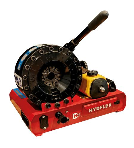
This workshop crimping machine facilitates the crimping of 1SN/2SN up to 25mm and 4SP hoses, up to 20 mm inside diameter. The bigger head opening without dies (68 mm) allows crimping a wide range of atypical fittings. The machine comes with 12 complete die sets ranging from 6 to 41 mm.
